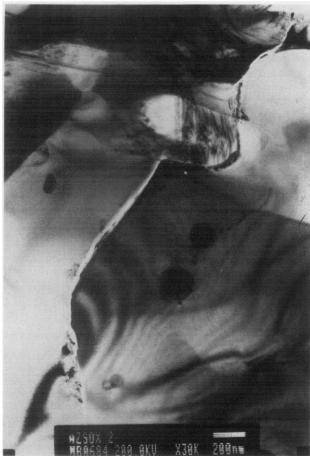
Fig. 9. Transmission electron micrograph of a sample deformed at 1673 K under stresses up to 100 MPa, showing microcracks at grain boundaries and along whisker interfaces.
